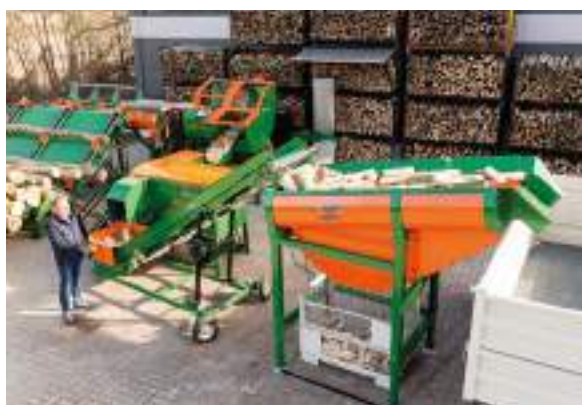
LogFix L waste wood is transported to a suitable container or an optional conveyor belt (image includes Option L).
